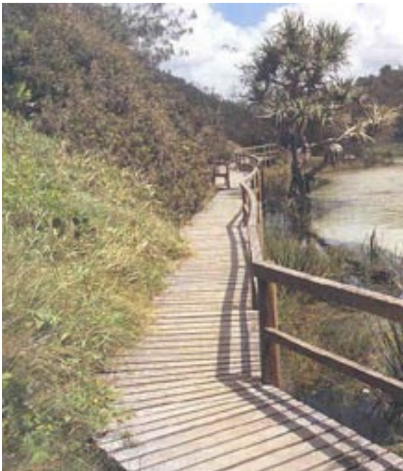
Observation deck and walkway utilises durable timber and non-corrosive fasteners.
