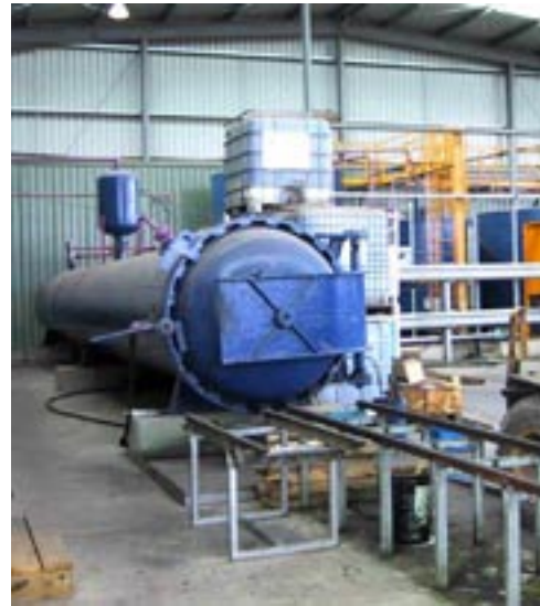
CCA timber treatment plant (Photo courtesy of Dr. Harry Greaves)
