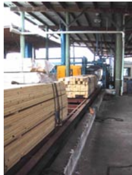
LOSP timber treatment plant (Photo courtesy of Dr. Harry Greaves)
